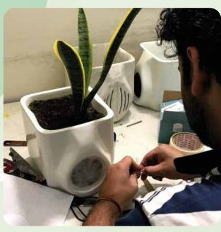
Breathing roots technology magnifies the air purification through plants by improving the breathability of soil. Superior hardware chassis design improves the air circulation through the internal system before passing on the contaminated air through soil-root zone. Once the air is treated by the micro-organisms around the roots, cleaner air is pushed out of the system.
